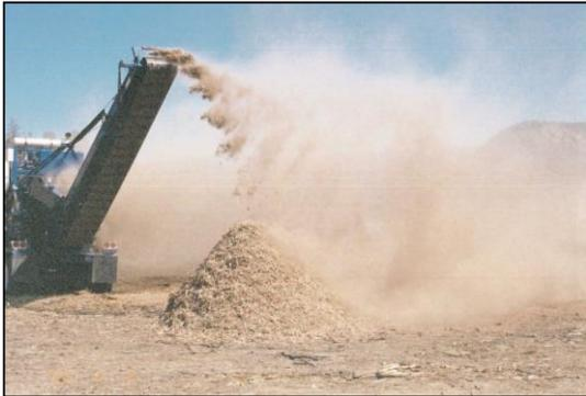
Grinder – Significant Visible PM Discharge
